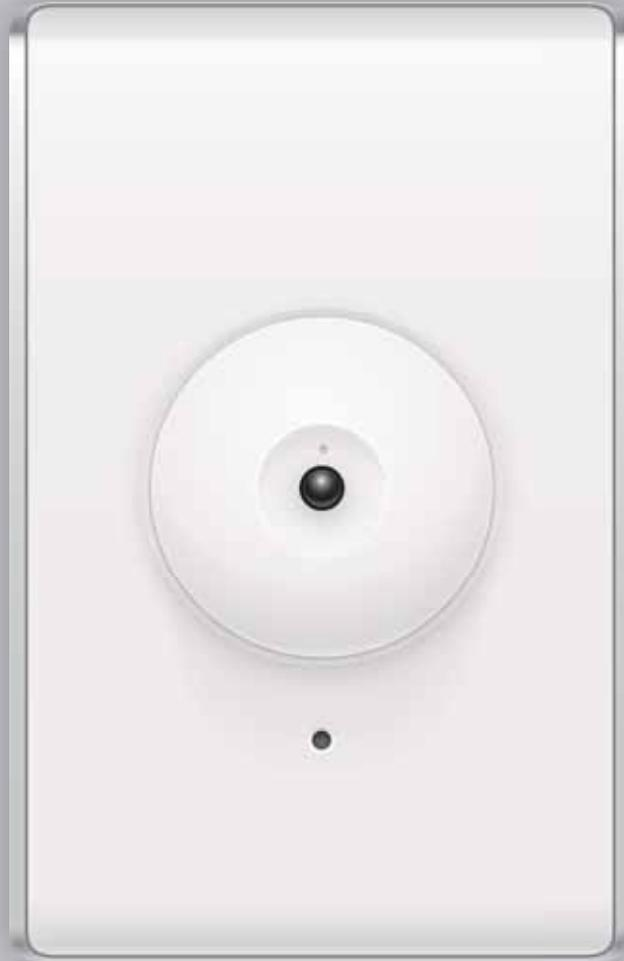
*The Camera System provides a crystal clear, real-time view of up to four areas inside or outside of your home. Discreet, adjustable cameras can display all the action on any TV, over the Internet, or on an LCD—even in low light or nighttime conditions. Each camera also includes a microphone, enabling audio as well as video monitoring.*
